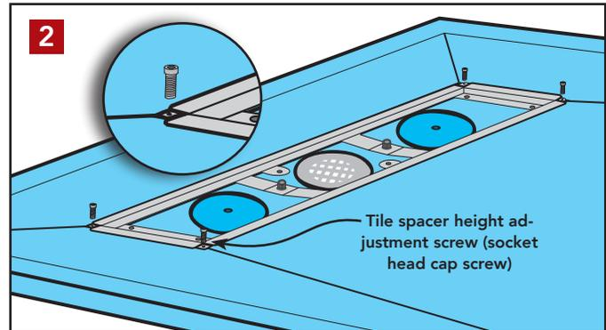
Insert a tile spacer height adjustment bolt into the threaded hole located at each corner of the tile adaptor. Identify these four bolts by their overall length: a bit over 3/4" (the longer bolts in the hardware kit). Turn the bolts until the heads contact the tile adaptor (use a hex driver if necessary).
