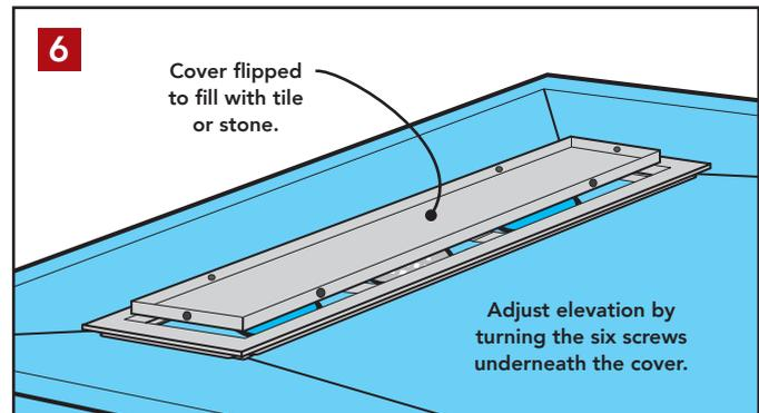
If you prefer to fill the cover, first rough-up its inside surfaces with 80 grit sandpaper, then clean them with a damp cloth. After it's completely dry, brush a coat of Tank/10® waterproofing onto the steel (to improve mortar adhesion). Use a modified thinset mortar to bed your tile or stone.
