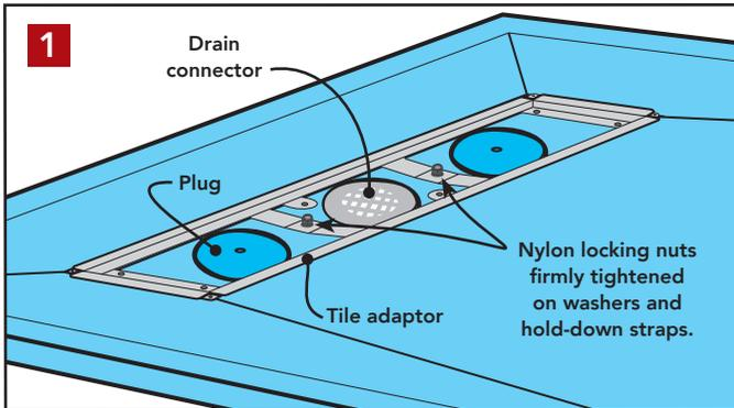
Place the tiling adaptor into the drain gully so that the hole in each hold-down strap slips onto a threaded stud in the gully. Slip a washer onto each stud and follow with a nylon locking nut. Tighten the nuts firmly to secure the tile adaptor to the gully floor.
