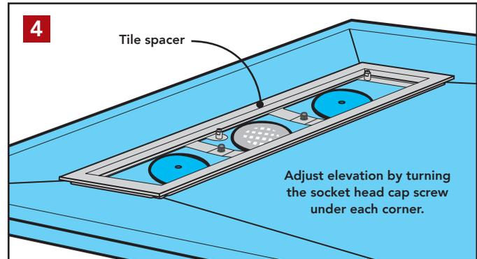
Set the tile spacer on top of the tile adaptor and height adjustment screws. When it comes time to tile, raise the tile spacer to the desired elevation by turning the screws below. You'll want to pack thinset mortar under and around the tile spacer once you have its elevation set.
