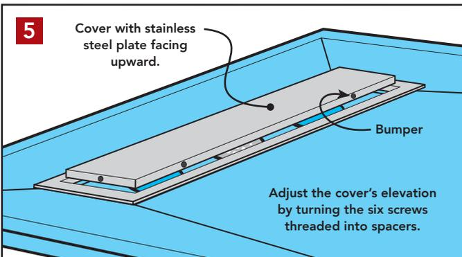
Press the six bumpers into holes in the edges of the cover (if needed, taper the bumper stems with a utility knife and add a drop of dish soap to insert them), then place the cover onto the spacers and height adjustment screws. Raise the cover to the desired elevation by adjusting the screws.
