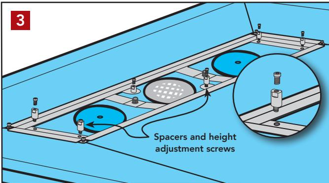
You can install the cover so it's on display, or flip it over and fill it with tile or stone. If you intend to show the steel, install spacers and height adjustment screws (3/16" long) in the six locations shown. If you plan to fill the cover, install only the height adjustment screws (no spacers).
